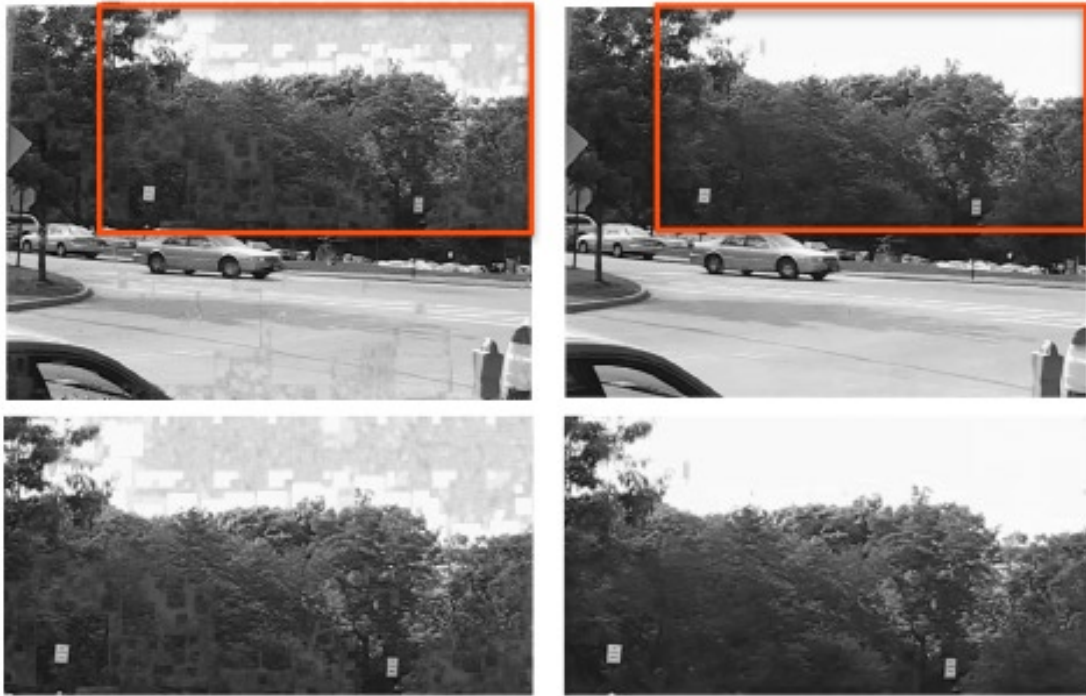
Figure 3.1: Reconstructed frame in a video at 40% compression. Left: Video Epitome [CFJ08], Right: Our approach. Below: Zoomed-in view of the red box. Our method improves reconstruction of both homogeneous and textured areas.
