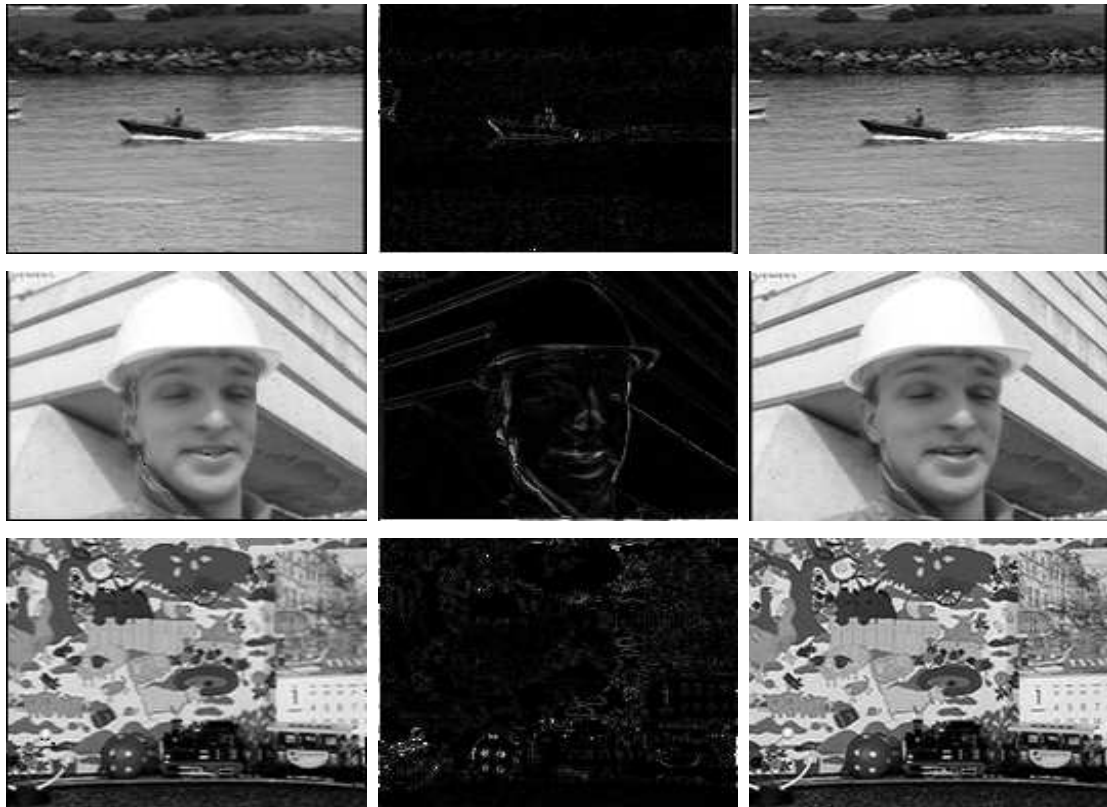
Figure 7.6: Qualitative results of our encoder. Predicted image using spatial, temporal and texture synthesis prediction modes (left). Residual error: black corresponds to zero error, white to large (center). Reconstructed video frames (right).
