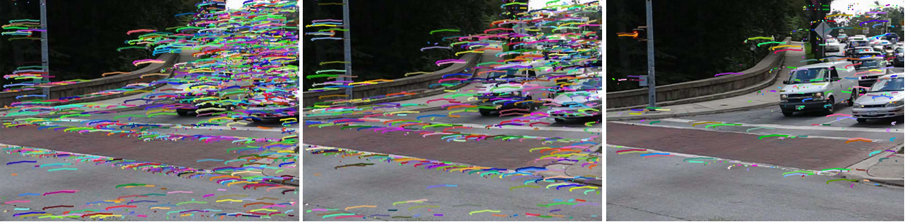
Figure 1. Varying the co-variant detection threshold produces different densities of trackable regions. There are typically three regions of interest, shown in the images. The tracks that persist through a wide a range of thresholds are typically the longest and most accurate.
