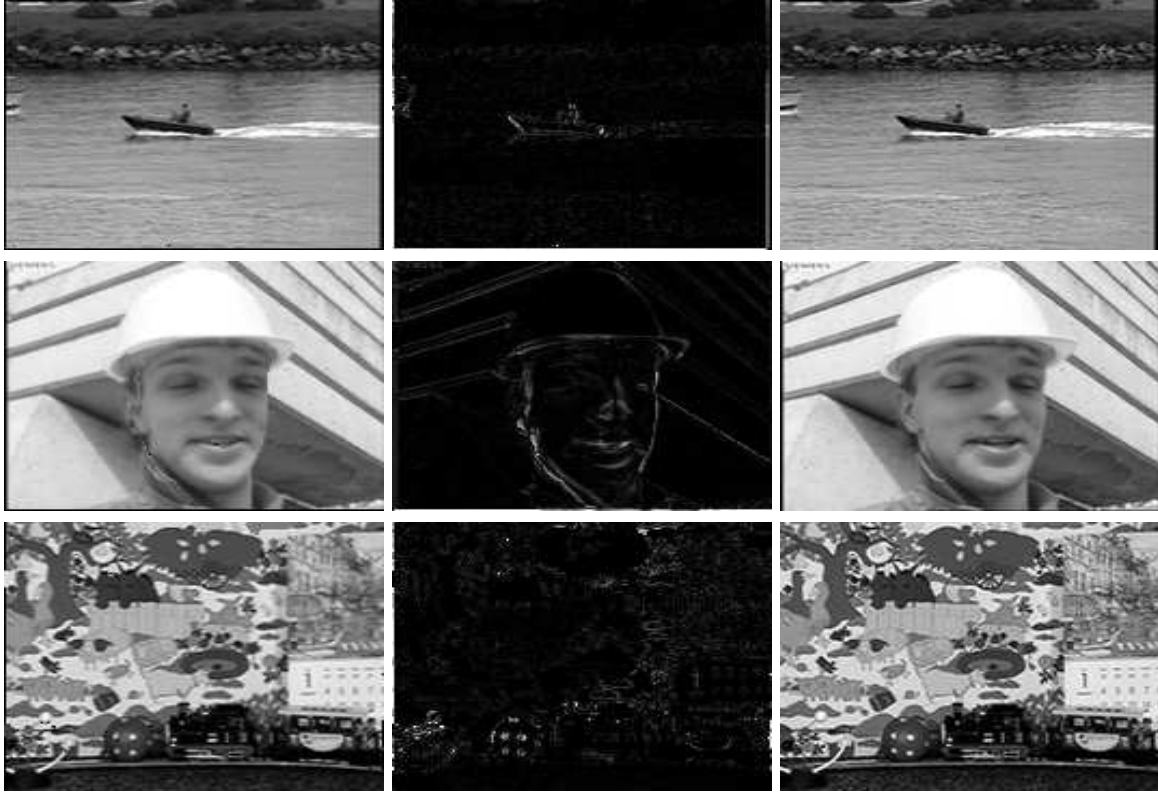
Figure 6: Qualitative results of our encoder. Predicted image using spatial, temporal and texture synthesis prediction modes (left). Residual error: black corresponds to zero error, white to large (center). Reconstructed video frames (right).
